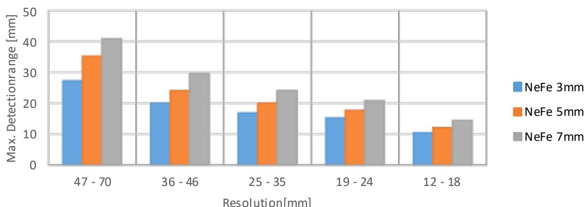
\* The data refers to the clear distance between test object and the upper edge of the sensor. The values are valid for the entire temperature range and for speeds from 6 to 300m/min.
